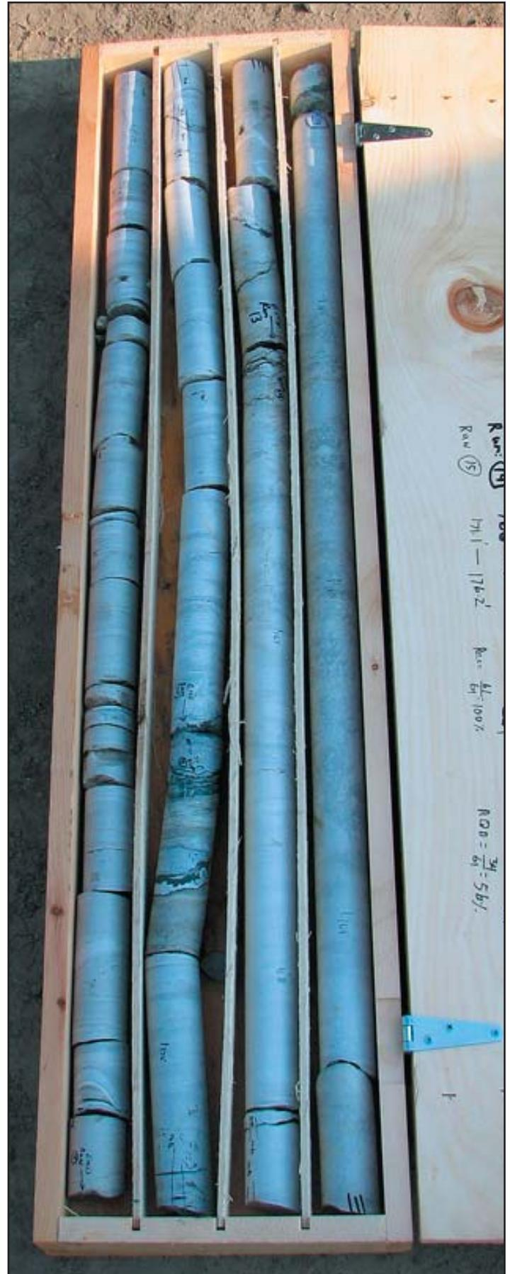
A selection of limestone samples from the Missouri side of the River, from about 160 feet below the water’s surface.
