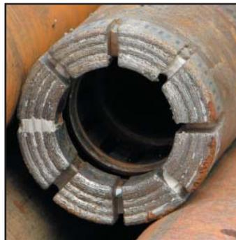
Geology crews attach this drill ‘bit’ to the drill to cut through the limestone bedrock of the river.
